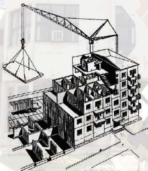
Large Panel Buildings of Slema 135 - Assembly in Progress
